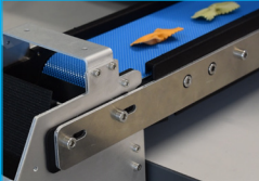
The SeedSorter fingers can be customized for different product sizes.
