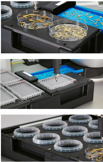
Different holders for cups, petri dishes or 96 well microtiter plates.
