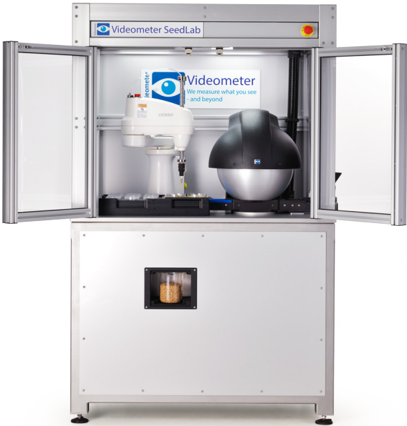
Different holders for cups, petri dishes or 96 well microtiter plates.
