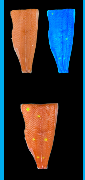
Detection of impurities in salmon with MSI tools (top left and right) and beamer projection (bottom).
