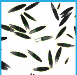
Classification of grass seeds - detection of weed seeds and foreign material.
