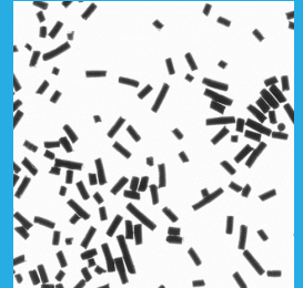
Segmentation of granules using backlight illumination
