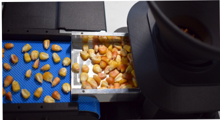
Even distribution of granules onto belt by vibration unit.
