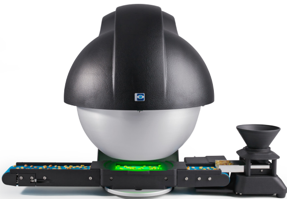
OSR (Oil Seed Rape)-application. Detection of admixture in OSR-samples.
