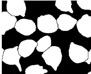
Touching objects are separated in segmentation process.
