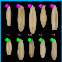
Oat de-husk application. Detection of husked and de-husked kernels.
