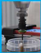
The pick and place robot detects each seed's center to sort and place it in its container. It can pick even the smallest seeds, like OSR.
