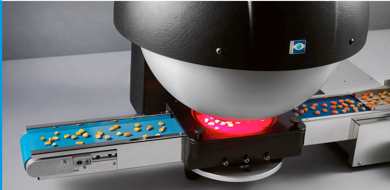
Maize (corn) application. Detection of healthy and defect maize kernels.
